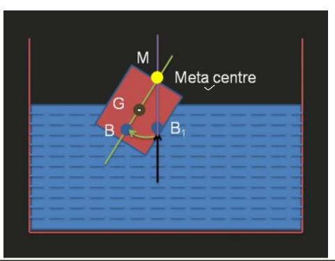
It can be also defined as an intersecting point between neutral axis line of the body and line of action of force of buoyancy.
