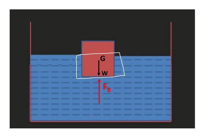
Whenever a body is immersed wholly or partially in a fluid then it is lifted up by a force equal to the weight of fluid displaced by the body and this Upward force is known as Buoyancy force
