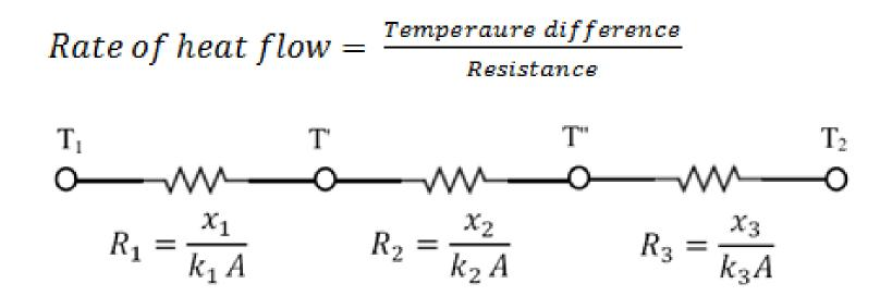
• The wall is composed of 3-different layers in series and thus the total thermal resistance was represented by R (=  $R_1 + R_2 + R_3$ ).
