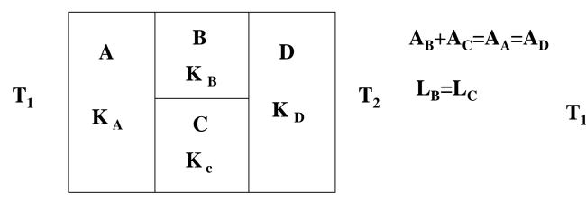
$$q_x = \frac{T_1 - T_2}{R_{tot}}$$
