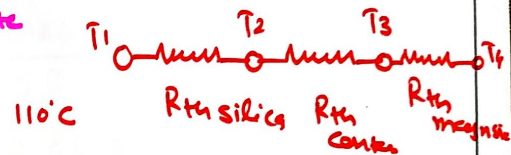
$$q = \frac{T_1 - T_4}{R_{total}}$$
