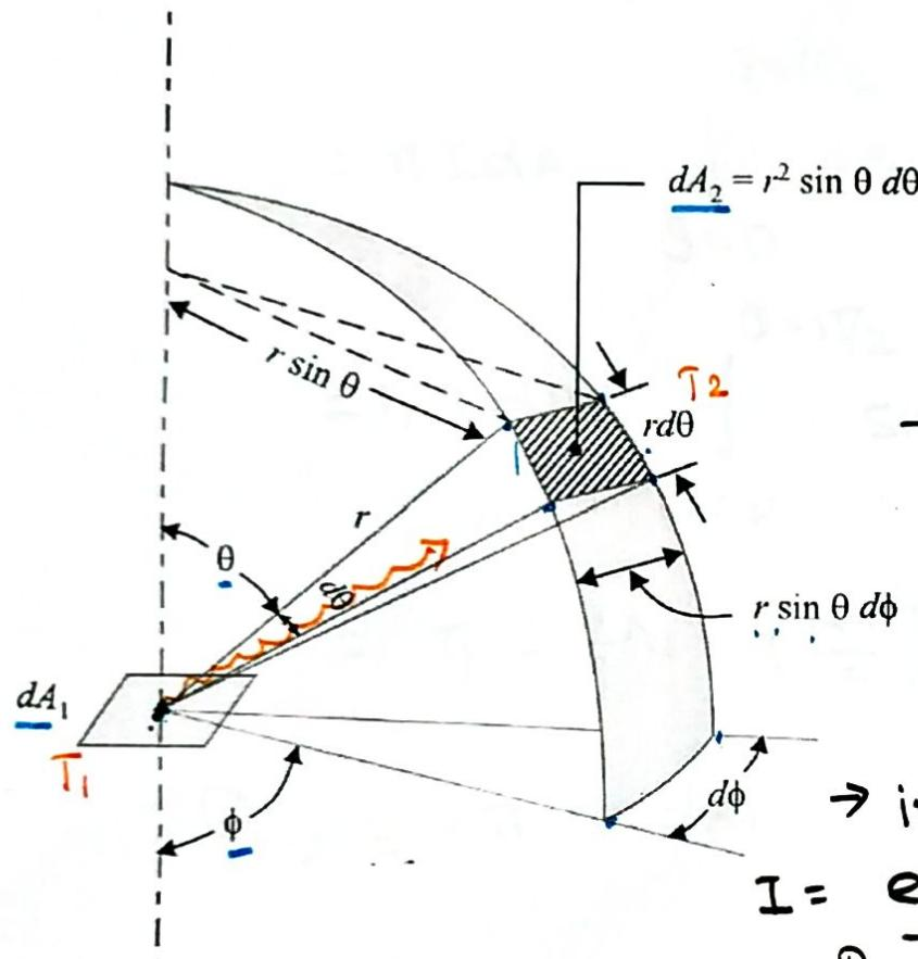
→ projected area of  $dA_1$  on a plane perpendicular to line joining  $dA_1$  and  $dA_2$
