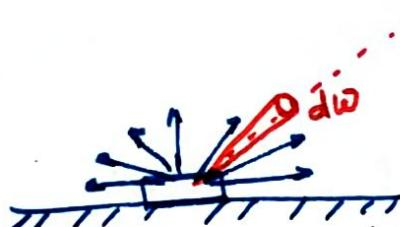
$$I_b = \frac{\text{energy emitted}}{\text{Power density} \times \text{Solid Angle}}$$
